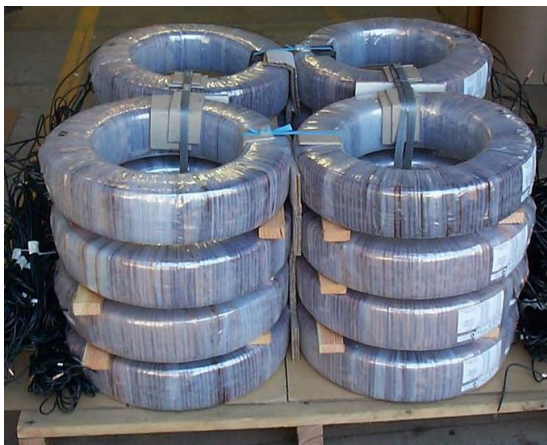
Fig. 3.5. A pallet of taped toroidal CTs. Reproduction permission requested from Stemar.
