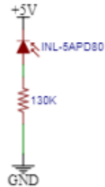
Fig. 4. Simplified schematic of the photodiode.
