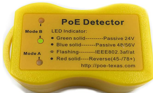
Figure 19: POE Detector Example
