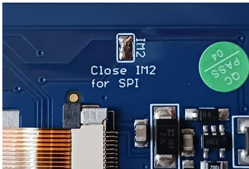
Figure 30: Touch Screen Breakout Board IM2 Jumper Connection for SPI Protocol
