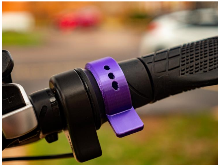
Figure 25: Picture of a thumb throttle on an e-bike (copyright pending)
