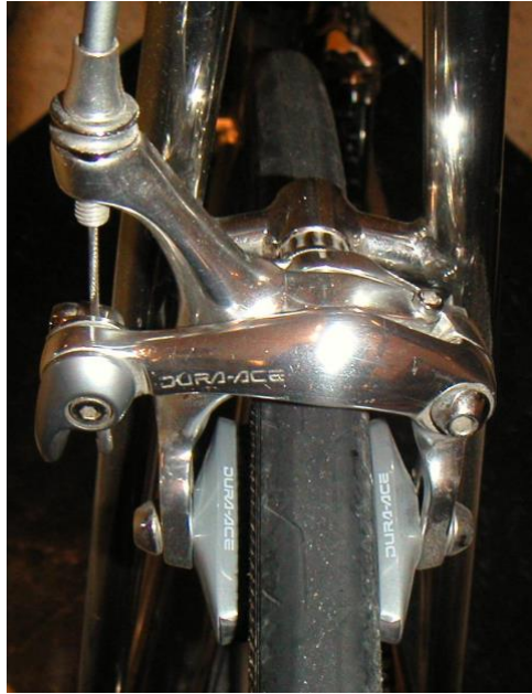
Figure 32: Dual pivot side-pull caliper brake
