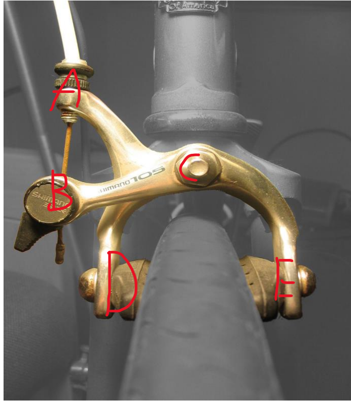
Figure 28: Single pivot-side-pull caliper brake
