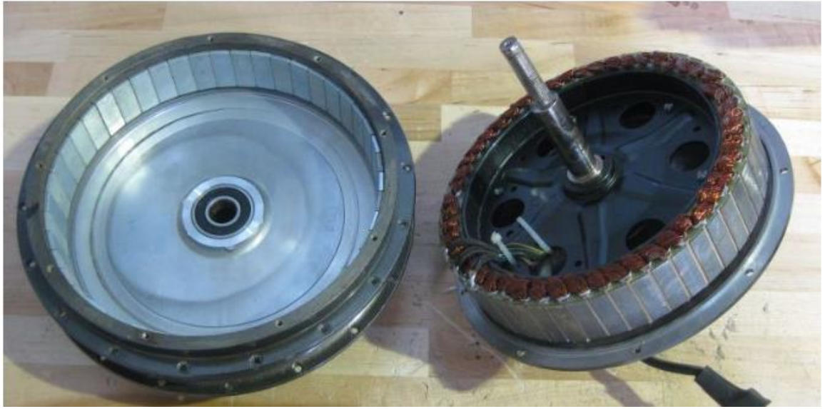
Figure 19: Direct Drive Motor (copyright pending)
