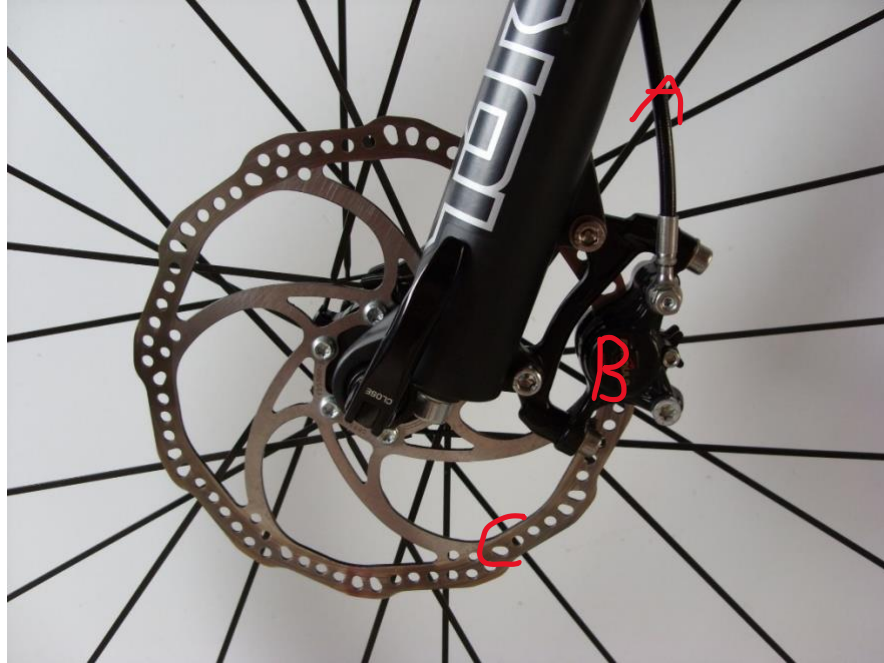
Figure 29: Hydraulic disc brake
