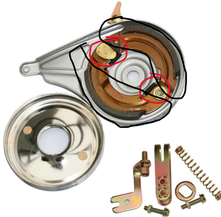
Figure 31: Internal of a drum brake
