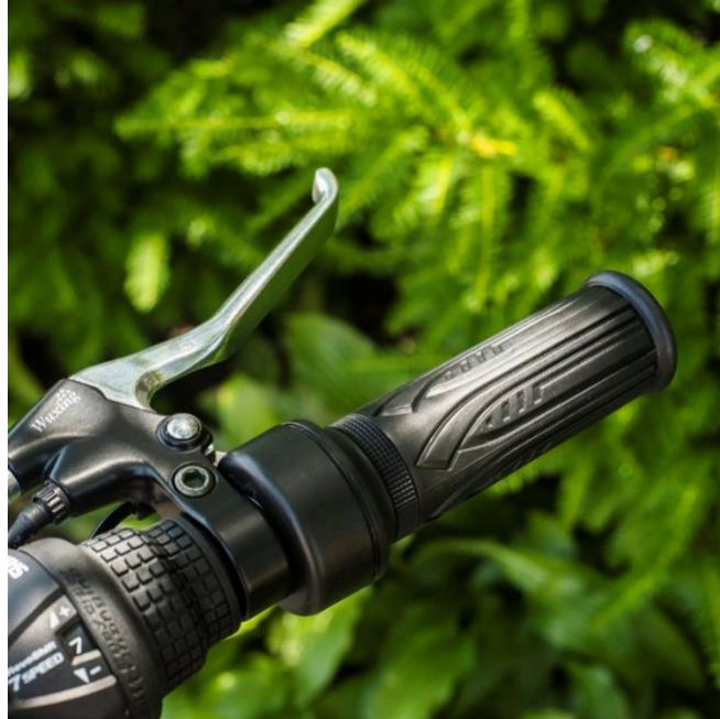
Figure 24: Picture of a full-twist throttle on an e-bike (copyright pending)
