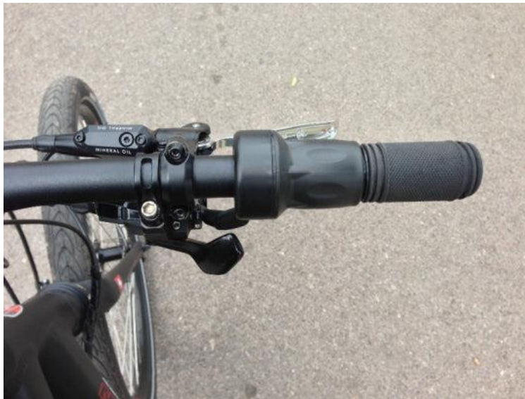
Figure 23: Picture of a half-twist throttle on an e-bike (copyright pending)
