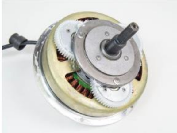
Figure 18: Geared hub motor (copyright pending)
