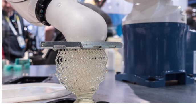
Figure 3.12 Example of how SLA printing can produce complex structures without support material needed. (Gustavo Rocha SI)
