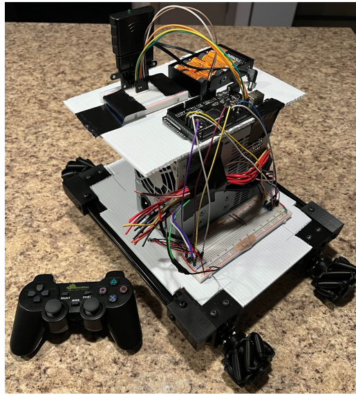
Figure 5.2: Prototype 1 Using a PC PSU, Arduino Mega 2560, a Lynxmotion PS2 V4 Controller, Greartisan 12V DC Motors, and Custom 3D Printed Mecanum Wheels Image taken by Cameron Nichols
