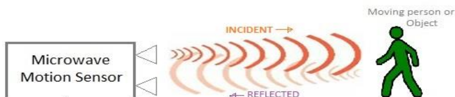
Figure 12 - Depicts the mechanisms behind microwave sensing
