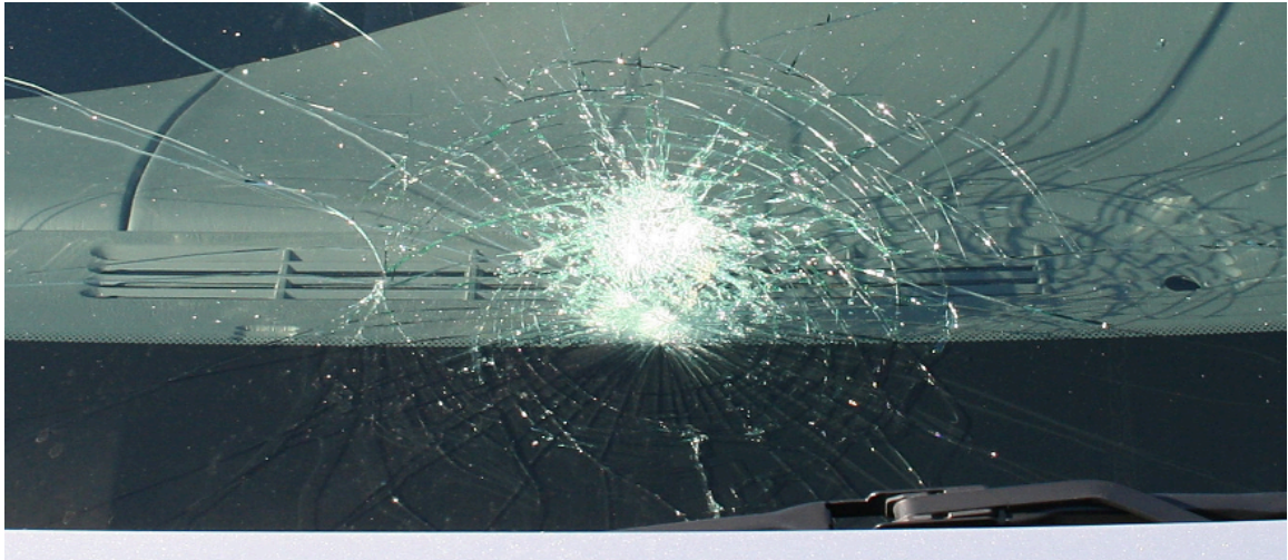
Figure 3.6.2.1: Automobile windshield with “spider web” cracking typical of laminated safety glass.
