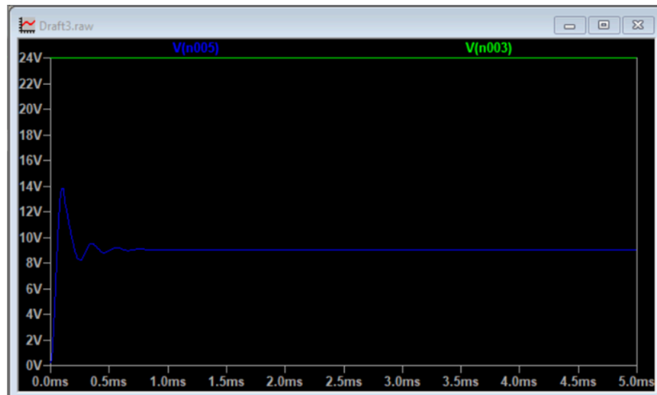
Figure 3.3.2.2: Buck converter simulation in LTspice. The green line is the input voltage, and the blue line is the output voltage.
