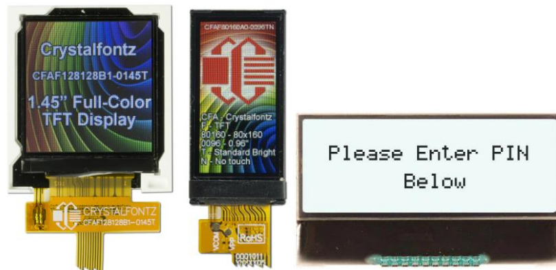
Figure 4 - Side by side Visual Comparison of Displays
