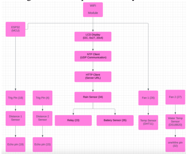
Fig. 3 Hardware integration block diagram
