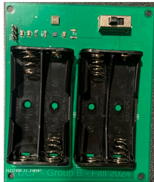
Figure 8.2.3 Complete Soldered PCB Top View (First Revision)
