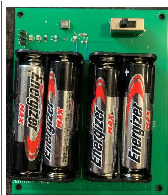
Figure 9.3.4 Corrected PCB With Battery Supply
