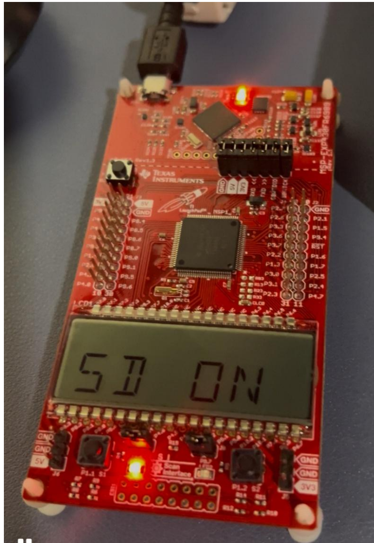
Figure 8.13: MSP-EXP430FR6989 during demo testing. Light turning on signaling 1 in binary encoding the letter N.
