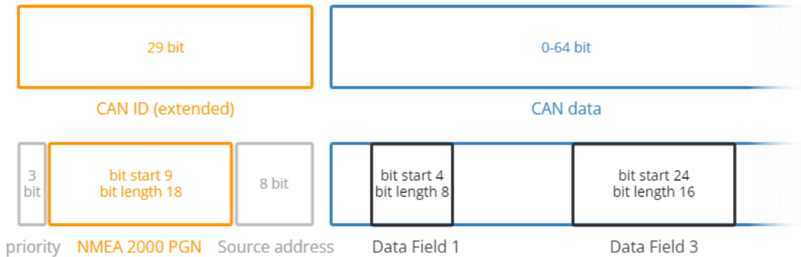
Figure: NMEA 2000 message (PGN and Data Fields)
