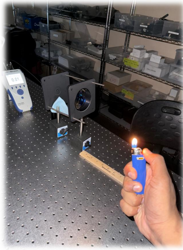
Figure 47. Experimental Setup for Characterization of power as a function of distance
