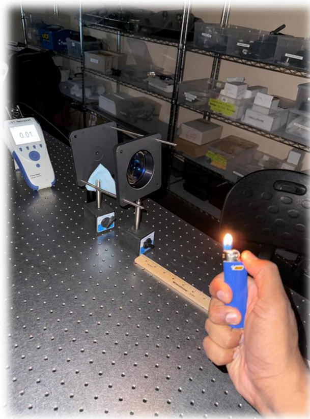
Figure 4946. Experimental Setup for Characterization of power as a function of distance
