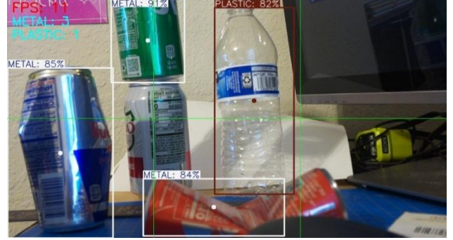
Figure 11: live object detection results using the deployed YOLOv11 model on Raspberry Pi, confirming real-time performance and high-confidence classification.
