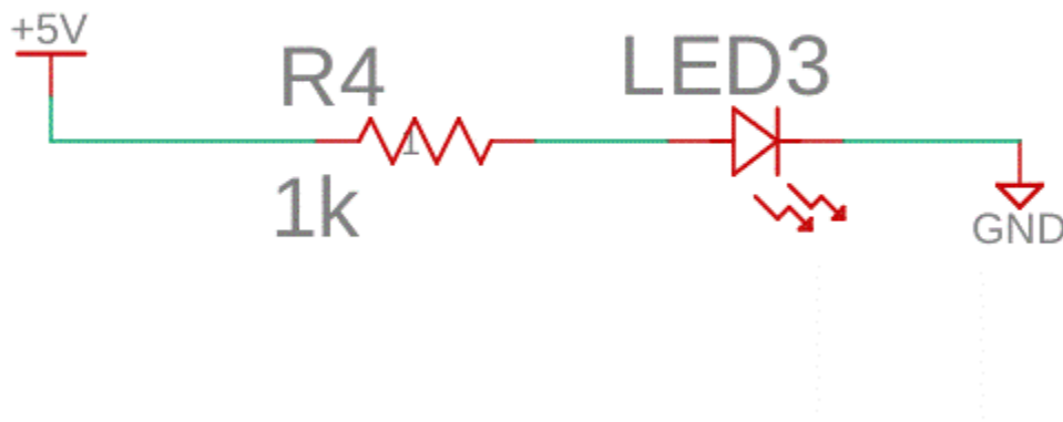
Figure 6.3.8 LED Implementation From 5V
