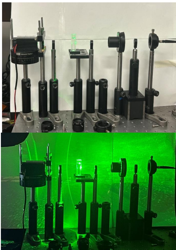
Figure 9.3.2 Successful Raman collection configuration
