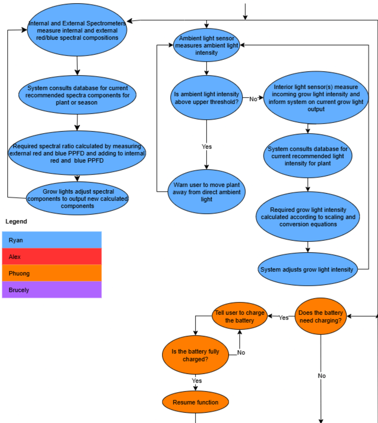
Figure 4: Continuation of the general system processes flowchart, this time focussing on optical systems and power management.
