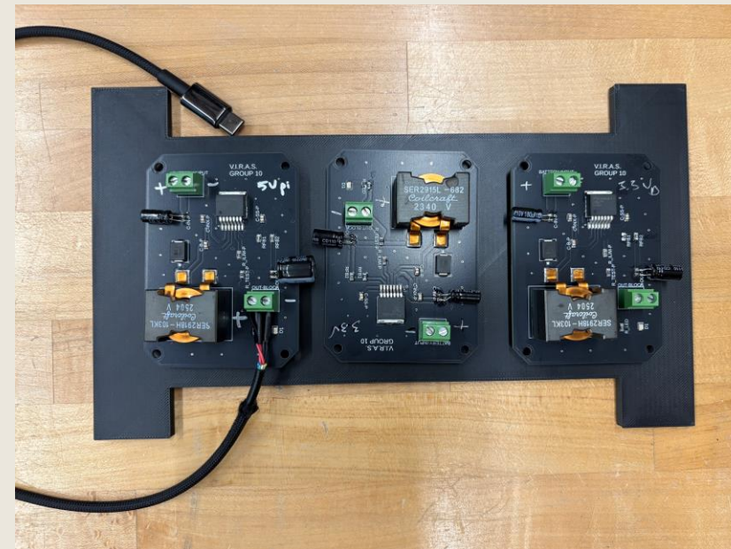
Power boards assembly
