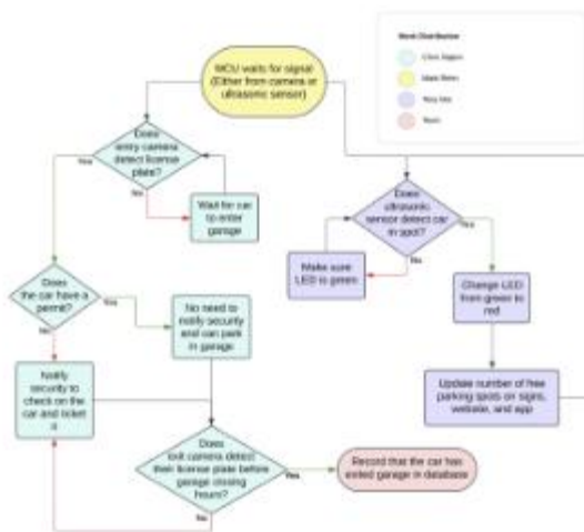
Figure 1: Parking Garage System Flowchart
