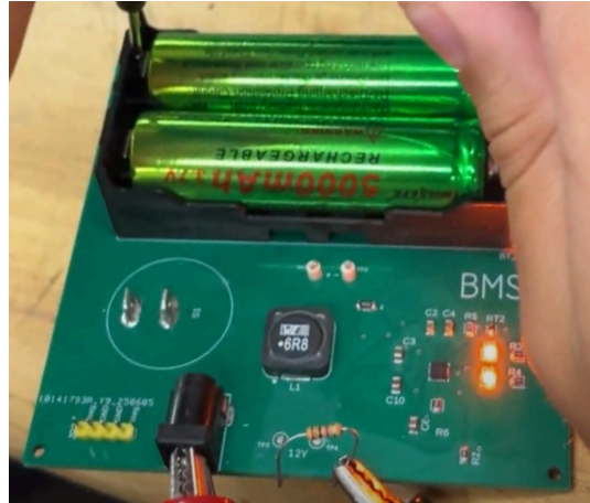
Figure 9.6 Battery Management PCB with Pulldown Resistor
