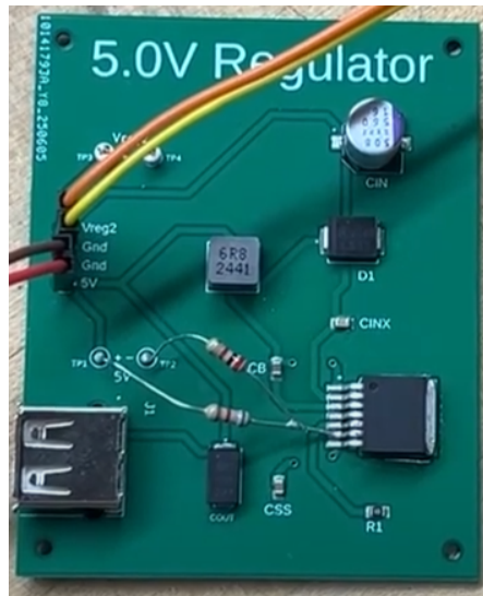
Figure 9.7 LM2679-ADJ Buck Converter with Voltage Divider
