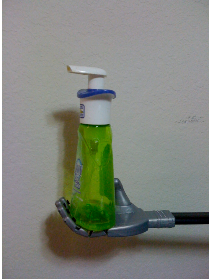
Figure 5.2.1.4: Graphical representation of Luke's hand executing testing procedure for grabbing a large object.
