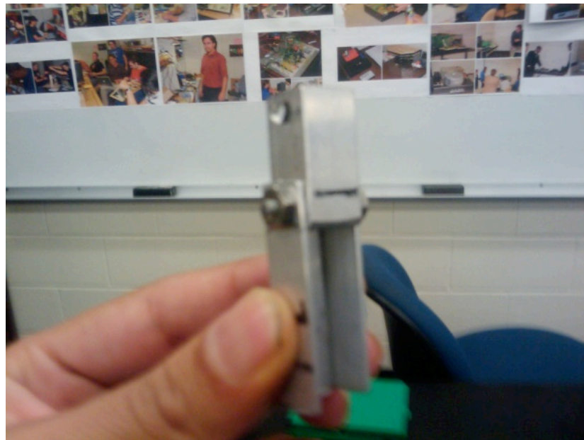
Figure 4.1.1.2: Finger with a single C-channel and two flat individual pieces complementing the other phalange.
