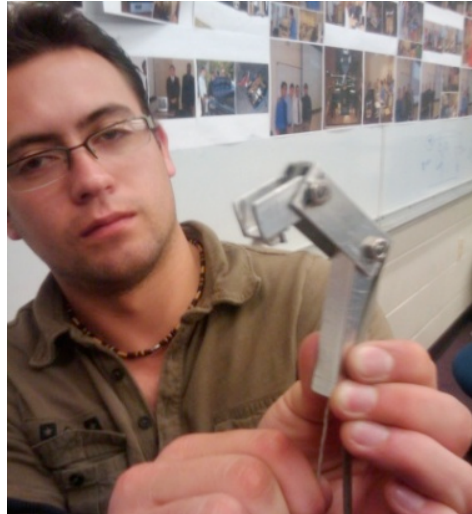
Figure 4.1.1.5: Finger with a rod and string attached to it implementing the tendon muscle mechanism.
