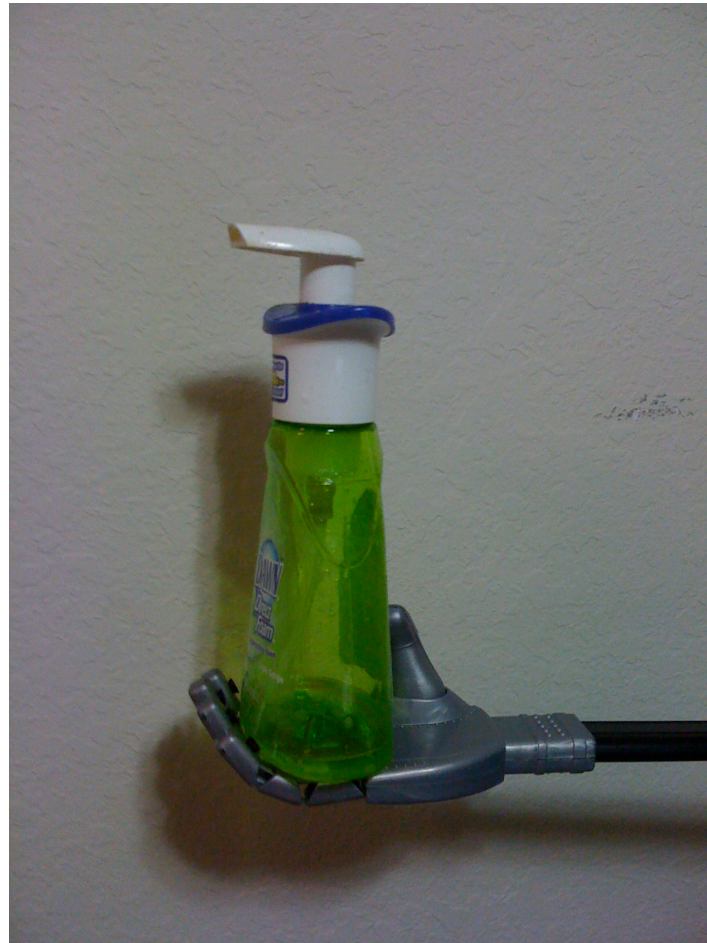
Figure 5.2.1.4: Graphical representation of Luck's hand executing testing procedure for grabbing a large object.
