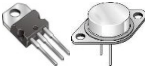
Figure 3.7.2.2: Types of IC Voltage Regulator Packages TO-220 and TO-3 "Photo Courtesy of Parallax Inc."
