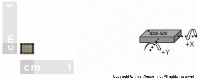
Figure 3: Integrated Dual-Axis Gyro (IDG-500) from InvenSense. Reprinted with permission from Sparkfun and InvenSense
