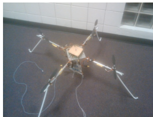
Figure 46: Aluminum prototype frame with close-up of central plate
