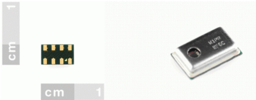
Figure 6: digital output barometric altimeter and pin configuration. Reprinted with permission from Sparkfun.com.
