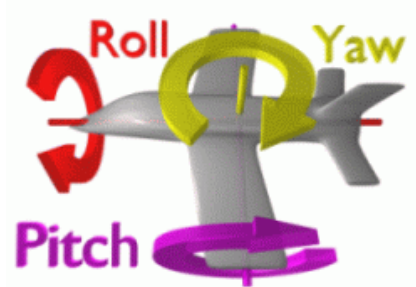
Figure 2: Visual representation of roll, pitch, and yaw. Reprinted under Wikipedia commons license, created by ZeroOne
