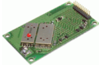
Figure 7: Ublox RCB-LJ receiver board; 71mm X 41mm. Reprinted from the Ublox RCB-LJ data sheet under non-commercial use.
