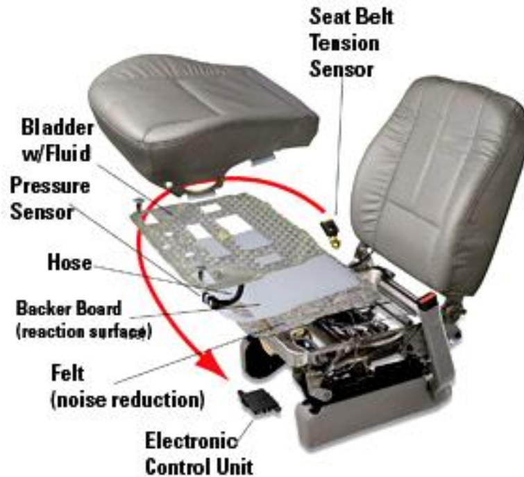
Figure 28: Delphi POD System Permission pending from Delphi
