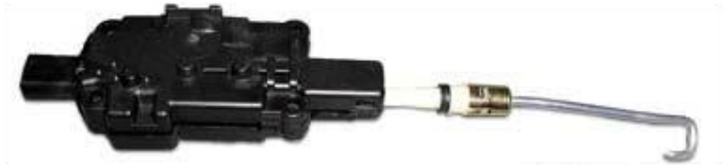
Figure 24: Door Lock Actuator Permission pending from howstuffworks.com
