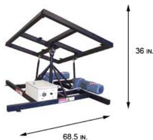
Figure 3.8.1(a) Standard units CKAS “T” Series 2DOF Motion Platform
