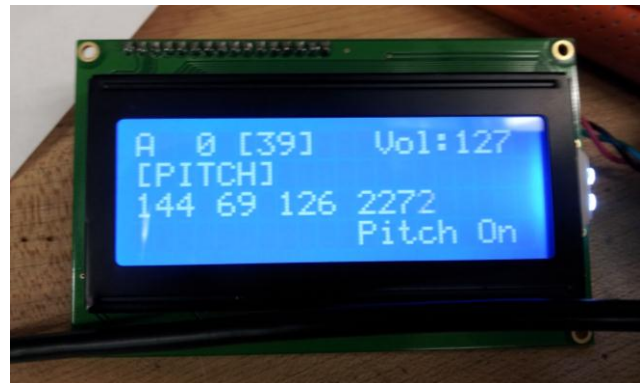
Fig. 7. LCD display demonstrating pitch mode and MIDI data
