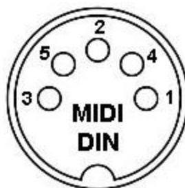
Figure 10: Standard MIDI 5-pin DIN pinout
