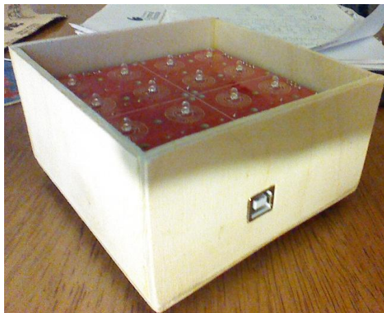
Figure 82: 4x4 prototype enclosure without faceplate
