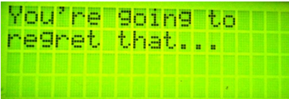
Figure 4.1.1.2-8: The LCD screen displaying the AI's opinion on the Player's move on the HMI 2 screen
