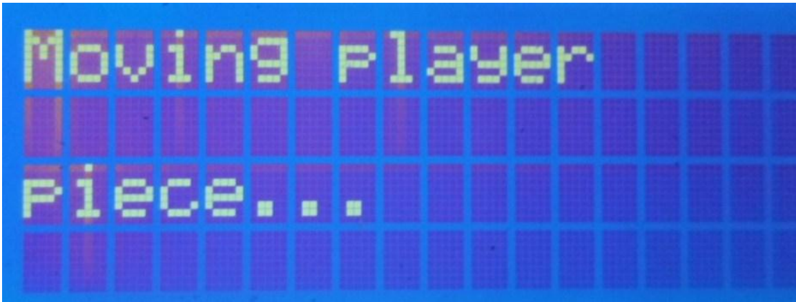
Figure 4.1.1.2-7: The LCD screen displaying that the Interactive Automated Chess Set is moving the Player's piece
