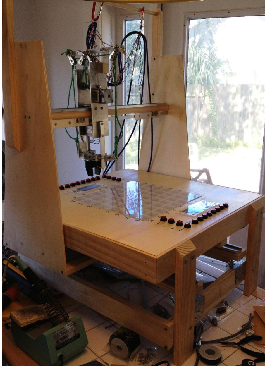
Figure 3.1-2: The full set up of our Interactive Automated Chess Set before the memory foam was attached to the claw prongs
