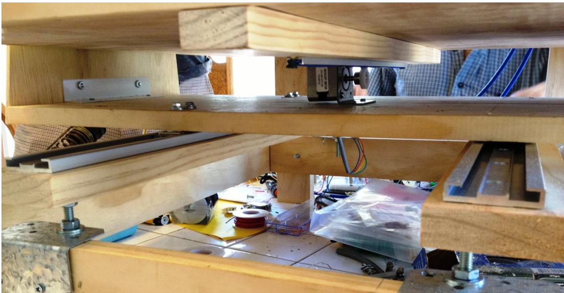
Figure 3.8-2: The gears and sliders located under the board that allow the A frame to move unimpeded.
