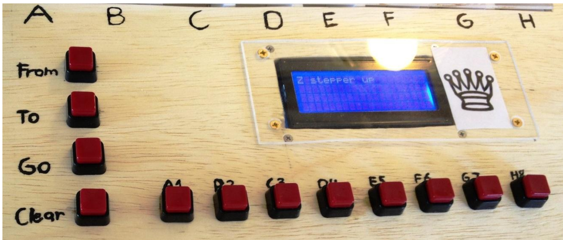
Figure 3.4-2: The actual HMI #1 panel and buttons for the Interactive Automated Chess Set
