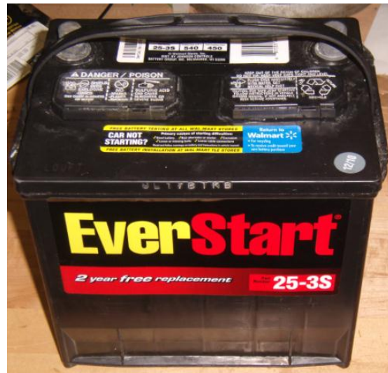
Fig. 6: 12 Volt Lead- Acid Battery
