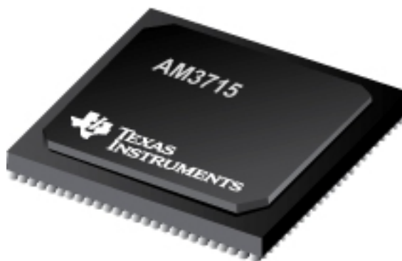
Figure 2.10: Texas Instruments AM3715 Sitara ARM Microprocessor
