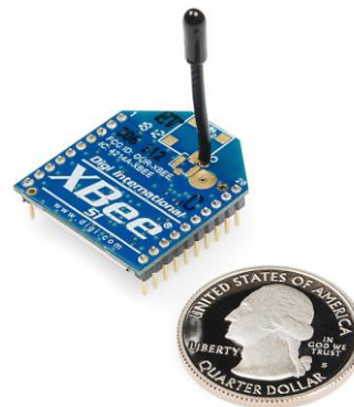
Fig. 4. XBee RF wireless module. Serves as the backbone of our project in that these modules are responsible for all our telemetry, including the transmission of sensor data, as well as command data from the base computer.
