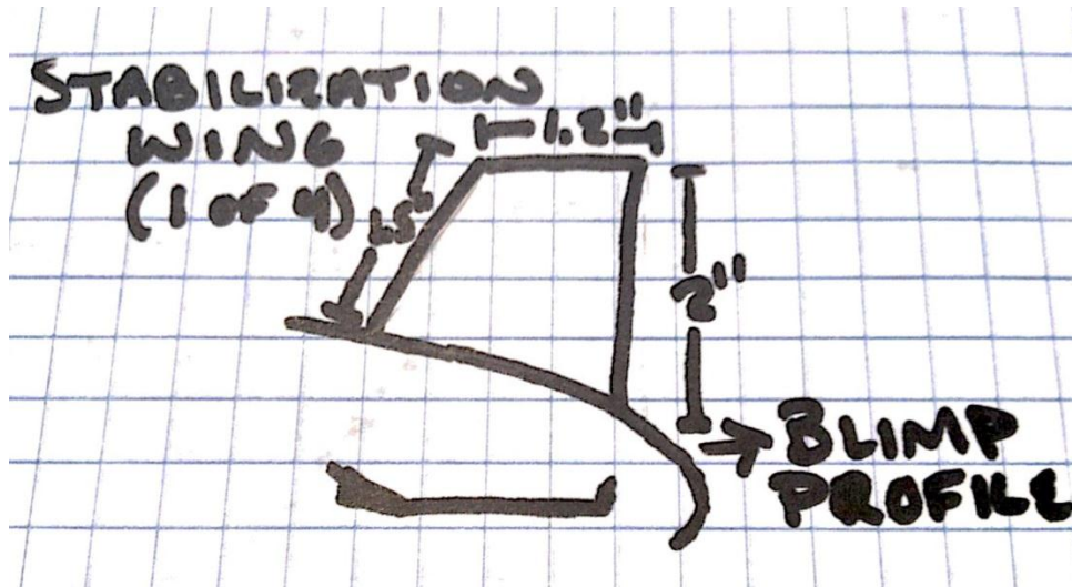
Figure 4.2.7: The figure above shows the top stabilizing wing. There will be four total; top, left, right, bottom.
