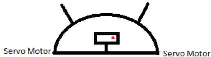
Figure 5.1.1: This is a zoomed in front view of how the camera will be kept in the camera stabilization system. Two Servo Motors will be able to turn the device in order to keep video still as blimp flies in the air
