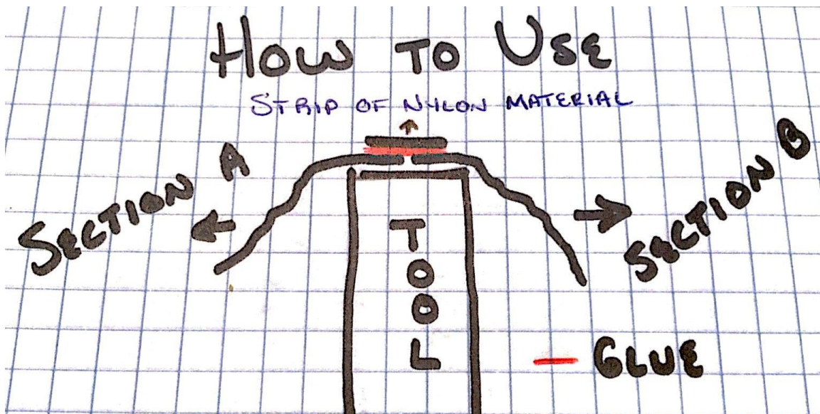
Figure 4.2.7: The figure above shows how we will use the tool. Put the two sections on the tool, stretch them out and then use the strip of nylon material with glue and mend the two sections together.
