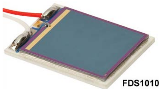
Figure 42: The Thorlabs FDS1010 Photodiode. The grey surface is the 9.7 mm width square active area
