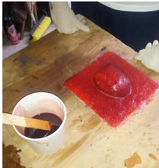
Figure 5: The fiberglass was placed on a wooden block shaped in the desired specifications for the handheld device.
