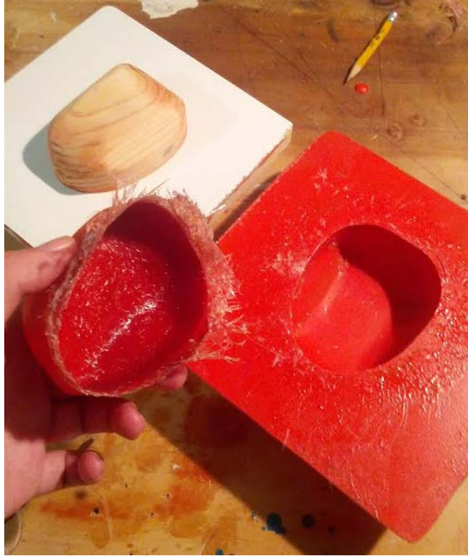
Figure 8: Depiction of all pieces used for making the mold possible. The only step left after this is to cut the edges straight and polish the case until it looks presentable.
