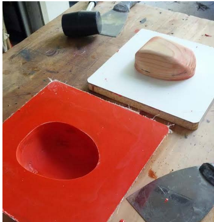
Figure 6: The fiberglass was then removed leaving the desired shape indented into the mold
