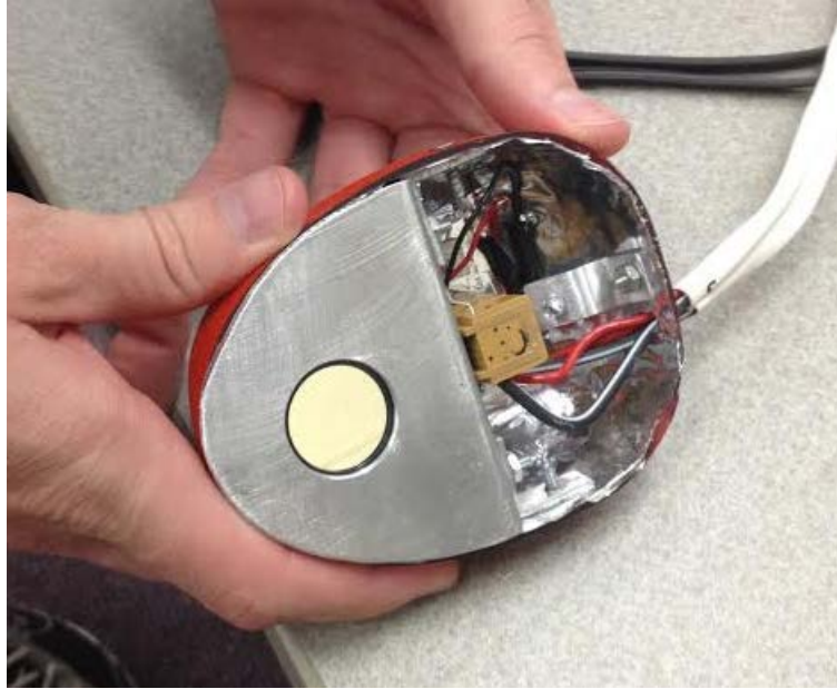
Figure 9: Bottom view of sensor case
