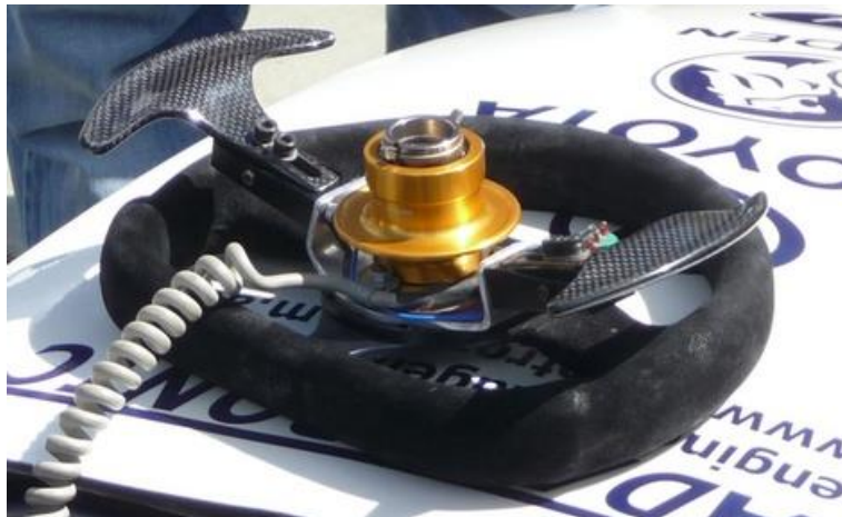
Figure 2: Electronic paddle shifter after setup and connection
