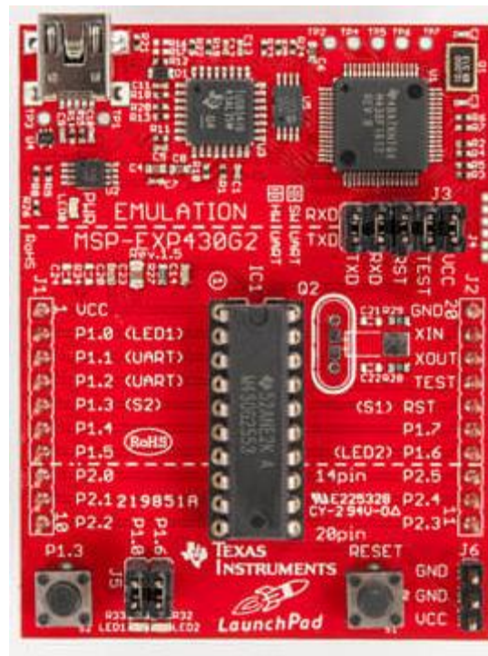
Figure 3.9.4. MSP430G2 in development board. [16]
