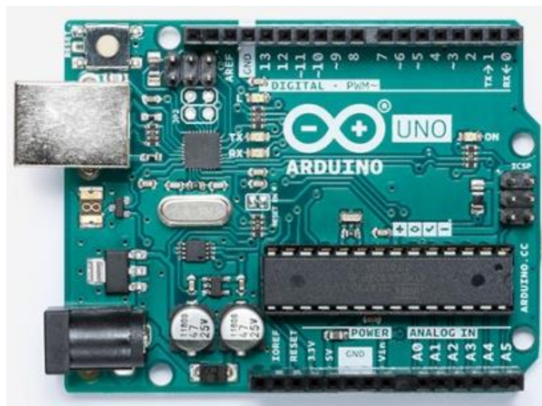
Figure 3.9.2. ATmega328/P in Arduino UNO development board [19]
