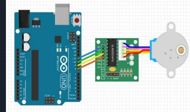
Note: The above image displays how we initially plan to use the Arduino to help in developing and testing the motor programming. ULN2003 breakout board will be recreated on PCB.
