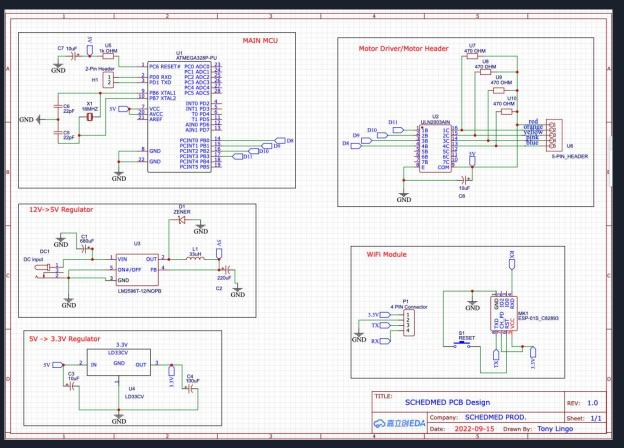
As the circuit of our design will change from a "programming state" to an "operating state", is important to make the proper adjustments for final PCB. Below is a display of SchedMed final schematic as it stands now.
