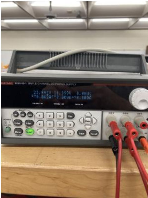
Figure 52: DC Power Supply Settings for Voltage Divider
