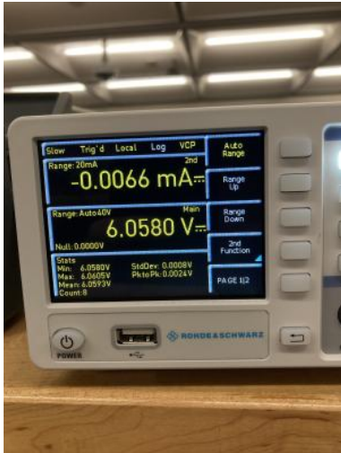
Figure 53: Multimeter Measuring Voltage for Voltage Divider
