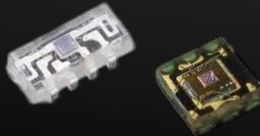
▶ Light Sensor (Left) Gyroscope/Accelerometer (Right)
