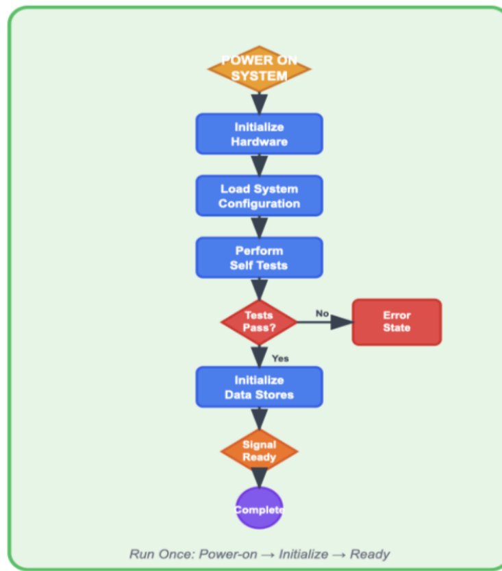
Figure 16: Central Control Unit Decision Logic Flowchart
