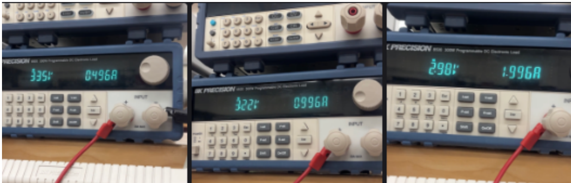
Figure 9.5 — 3.4V Regulator Testing
