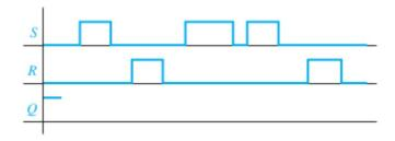
**11.12** Using a truth table similar to Figure 11-8(b), confirm that each of these circuits is an S-R latch. What happens when S = R = 1 for each circuit?
