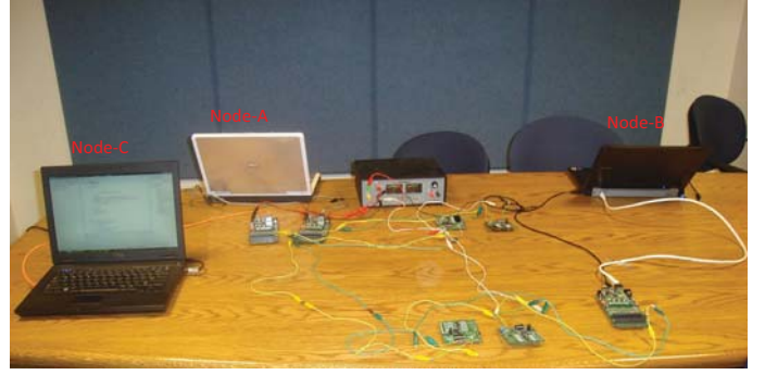
Figure 4. Prototype Setup: Three nodes, Node-A sends file to both Node-B and Node-C
