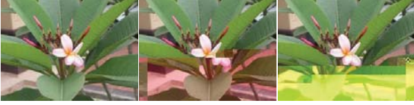
Figure 7. Original image file and received image files for image file transfer in full duplex mode. The very left picture represents the original image file and following images are received images at Node-B and Node-C accordingly.
